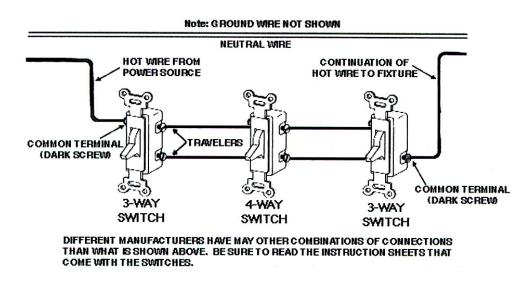
The schematic drawing below illustrates how the contact points within the switches can route the electricity to the light fixture:
