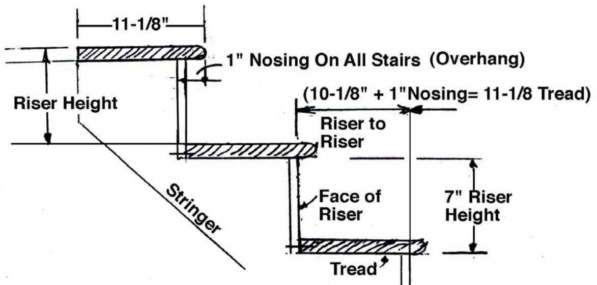
Your first step, then, is to measure the total height of your steps, from the footer up to the level of your landing deck. Divide that figure into equal increments, so that you end up with a step height between 7" and 8". Remember that the last "step" will be from the top tread up to the landing; for a 28" height, for example, you'd build three 7" steps.
