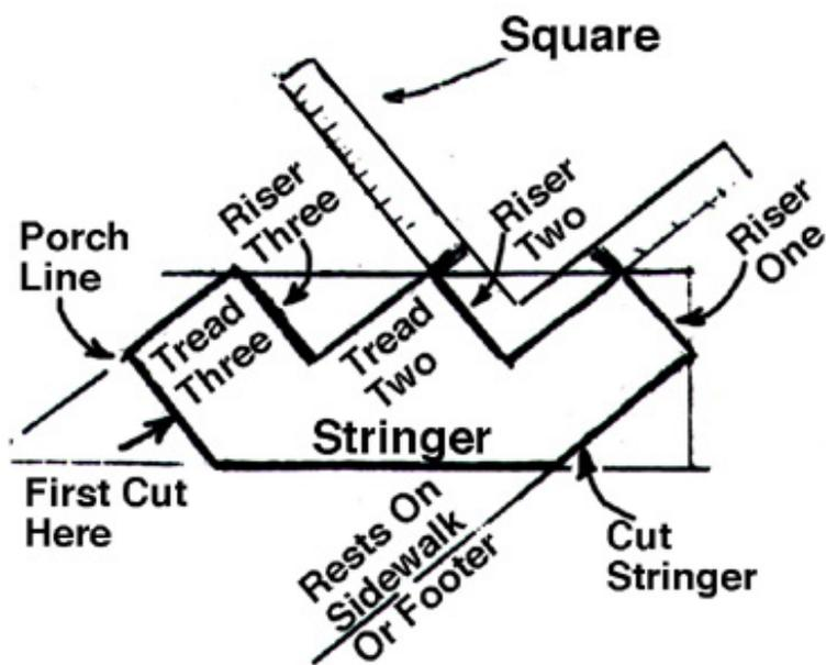
Now, before you cut, STOP, THINK, and CHECK YOUR MEASUREMENTS to make sure you have treads and risers of the right dimensions. Then, cut out the stringer. (You can use a circular saw for most of the cut, but you'll probably need to finish off the inside corners with a hand saw.) When you've cut your first stringer, use it as a pattern for the other(s) you'll need.
