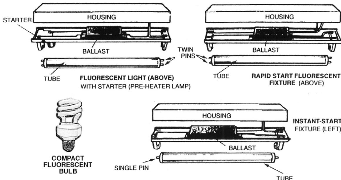
A **hard-wired fluorescent fixture** must be polarized to the circuit. That means the black wire on the ballast must connect to the hot wire of the lighting circuit (usually a black wire), and the white wire on the ballast must connect to the neutral circuit (white) wire. The fixture housing should be grounded for the fixture to light reliably.
