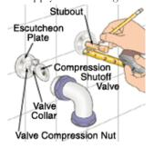
short would be disastrous – you might even allow a little extra length. On the other hand, the supply stop handles should not extend more than 3" from the wall when open.
