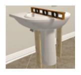
sink and the floor on either side of the pedestal.) If the parts move too much when you are positioning them, use plastic shims under the pedestal to keep it from rocking and foam pads under the sink bowl to level it, before marking the position of the mounting holes on the wall. After you have completed the installation, you can fill any gaps at the floor or between the sink basin and the pedestal with silicone caulk.
