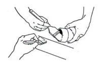
3. Apply primer to the inside of the pipe and the outside of the fitting, and allow to dry for a few minute. Then, brush on the PVC cement.
