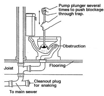
If the trap is clear, but the waste and water don't seem to move through as they should, then there's another possibility to consider. Instead of a clog in the outflow path, water may not be able to flow into the stool rapidly enough to start the flush process. The most common symptom of this problem is that the water rises up in the bowl, and then slowly lowers without swirling.
