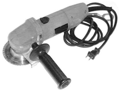
4-1/2" angle grinder w/ diamond masonry blade
