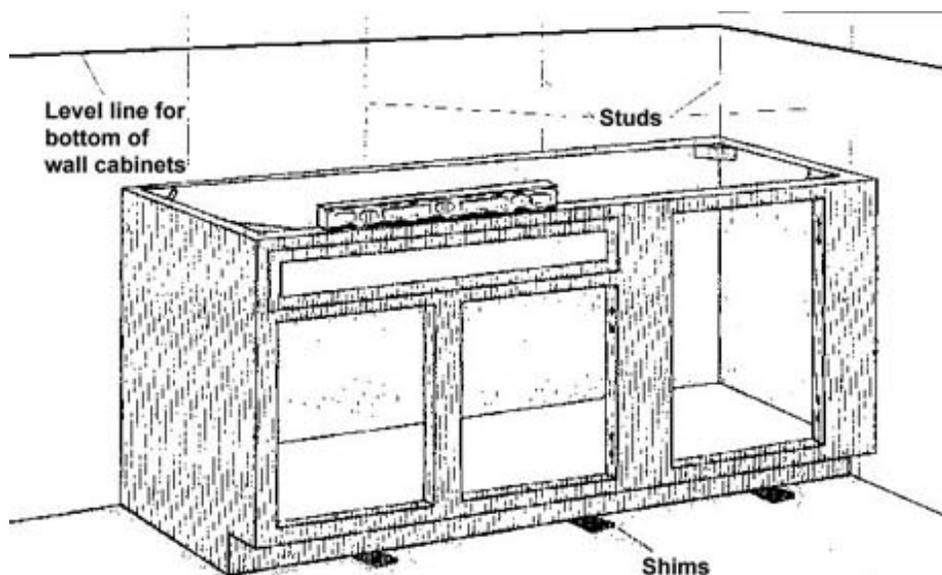
It usually works best to assemble all the cabinets for one wall on the ground, attaching the cabinets to each other before mounting them on the wall as a single unit. Remove the doors and any loose shelves; then, align the frames and use C-clamps to hold them together while you screw each cabinet to its neighbor at the front, at both top and bottom, using 2-1/2 inch panhead screws
