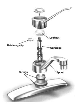
On a cartridge faucet, pry off the decorative cap and remove the screw underneath; then, lift off the handle and the handle body, a cylindrical slotted fitting. Before removing the spout, you'll need to unscrew the round retaining nut on top of it.
