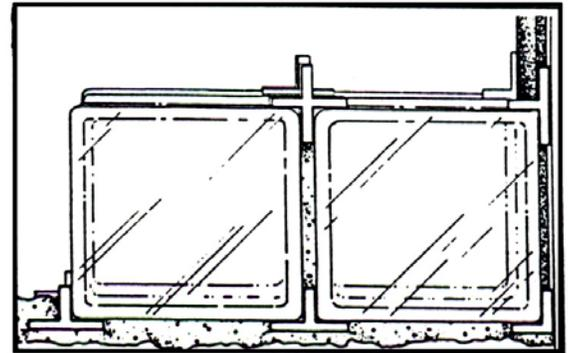
Once the panel has been assembled and the joints tooled, allow the mortar to set for another 15 - 30 minutes. Then, clean off any excess mortar from both sides of the panel and fill in any voids in the joints. If you used spacers, break off the projecting ends, leaving the body of each spacer imbedded in the mortar. After you have done all this, clean off any remaining mortar from the face of the bricks and let the panel set overnight for the mortar to harden.
