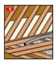
**Cellulose** (and other loose-fill) insulation can also be installed in an attic without flooring. While it's easy to just pour the insulation into the spaces between the joists, you may wish to rent a blower, as it will "fluff-up" the material uniformly, leaving no dense lumps. Install the insulation into each and every joist cavity, making sure you have filled the space completely. Contractors will often "shoot" in material to a depth of more than twelve inches, to allow for some settling.
