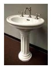
Most of today's sinks are made from vitreous china, a glass-like porcelain, and are available in many sizes, styles, and colors. Be sure to open the box and inspect the parts when you first bring them home, so you can replace any damaged pieces before you're ready to put them in place. Since three different faucet hole placements are common in pedestal sinks, make sure that the sink and faucet you choose have the same hole arrangement.
